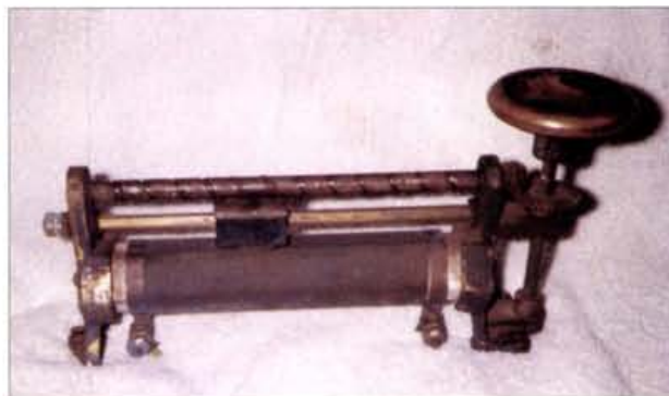
Fig. 4: A 'macro' volume control! Peter GW4OZU says that this large surplus variable resistor still has 'War Finish' clearly marked on one end.
