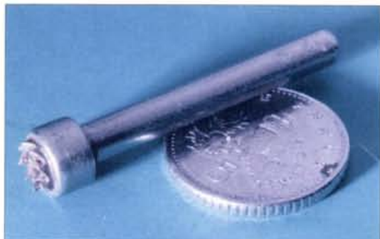
Fig. 1: Cutting 'islands' made easier with this cutter from Peter Crabtree G7TOO. (See text for details).
