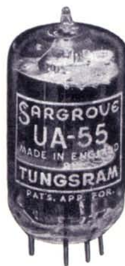
Fig. 3: Actual view of a Sargrove UA-55. Note the B9A type base.
