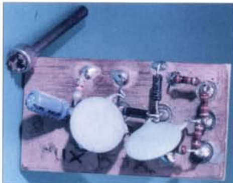
Fig. 2: A project showing how neat the results of using the cutter can look in practice.
