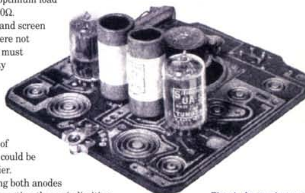
Fig. 4: An early type of 'printed circuit' receiver using two Sargrove UA-55s.
