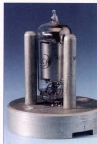
Fig. 9: The answer to the picture conundrum is - it's a valve pin straightener!
